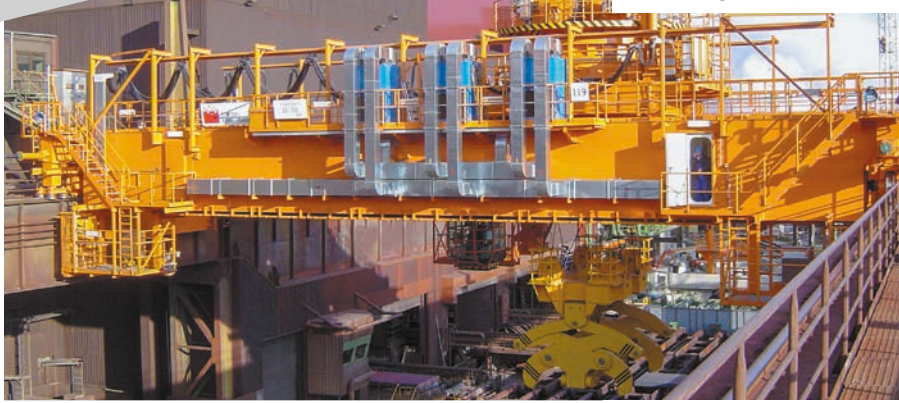
Ladle Transport Crane 390/60t x 40m
